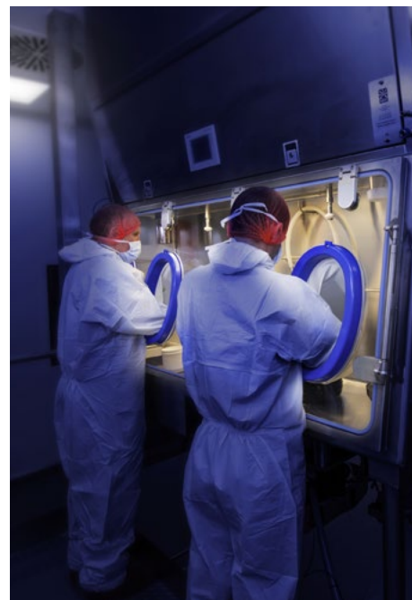
API Isolator at the Tredegar, UK site Specifically designed to provide operator protection and control of airborne contaminants generated whilst manually dispensing active potent compounds.
